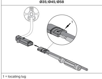
Plug the **dead** connecting cable into the angled plug until the locating lug clicks into place in the angled plug. If necessary, use a suitable flathead screwdriver to assist with insertion. Set the screwdriver into one of the two grooves on the plug-in connecting cable provided for this purpose.
