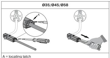
Insert a suitable flathead screwdriver right into the recess of the locating latch, so that the latch releases the locating lug from the plug.
